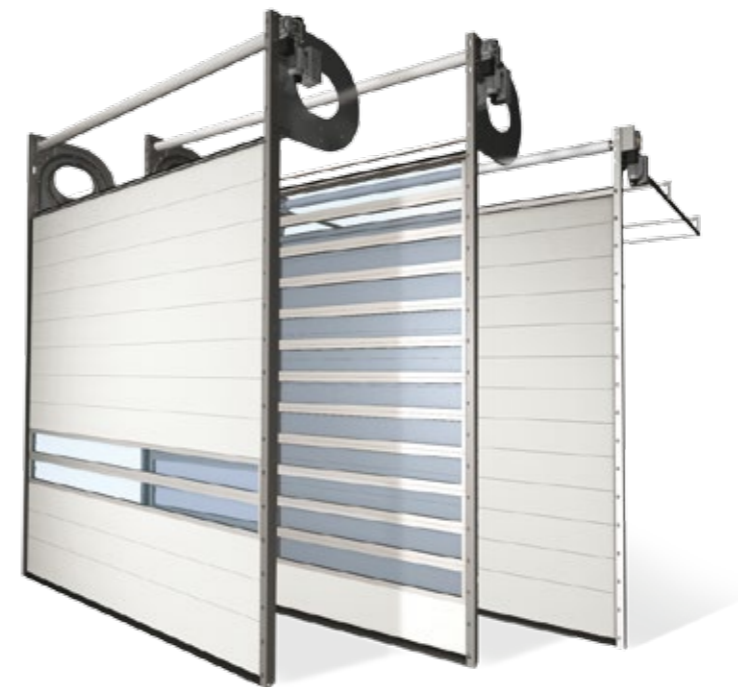
U-value Helix/ S600 ISO 40 mm sectional door: 5,000 x 5,000 mm: 1.77 W/m 2 K U-value Helix/ S600 ALU 40 mm sectional door: 5,000 x 5,000 mm: 4.25 W/m 2 K
